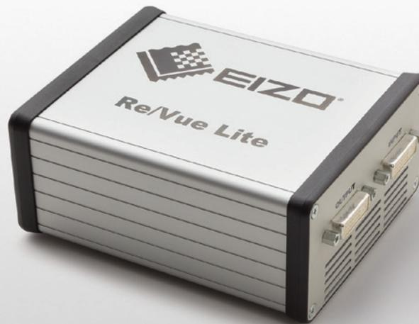
The Re/Vue Lite supports resolutions of up to 1920 × 1200 from both digital and analog sources. It provides cost effective video encoding and streaming to connected monitors for ATC and C2 markets with mission-critical redundancy.
